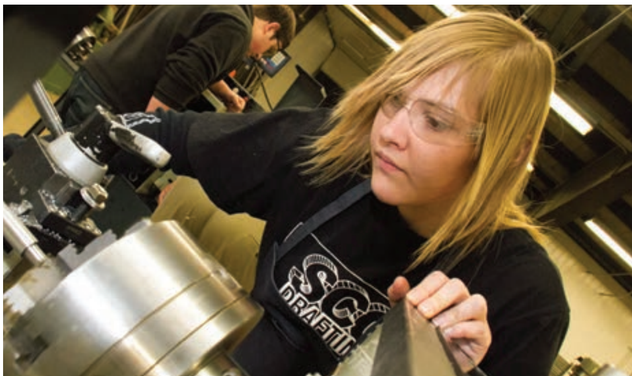
Student at Southeastern Community College working on a lathe, which is used for shaping wood, metal, or other materials.
